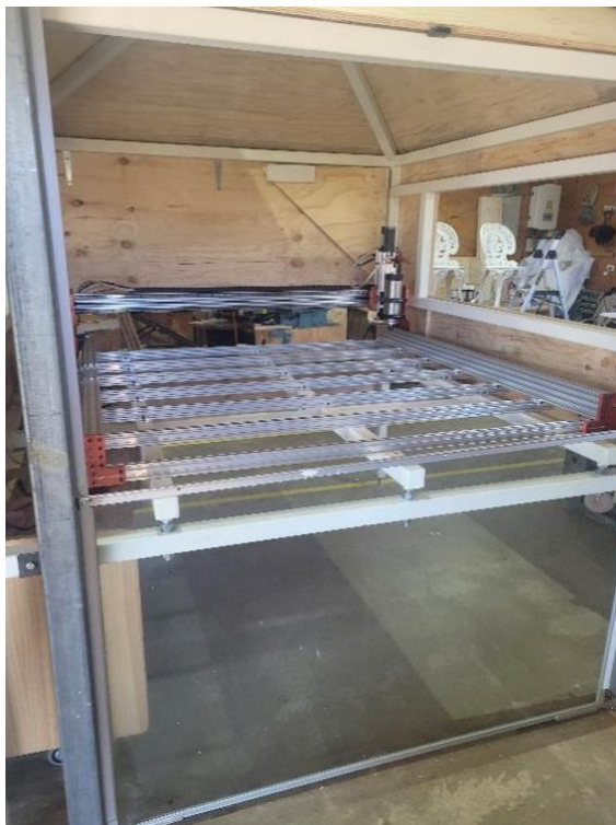
The CNC Router Bed It can hold a sheet of plywood
