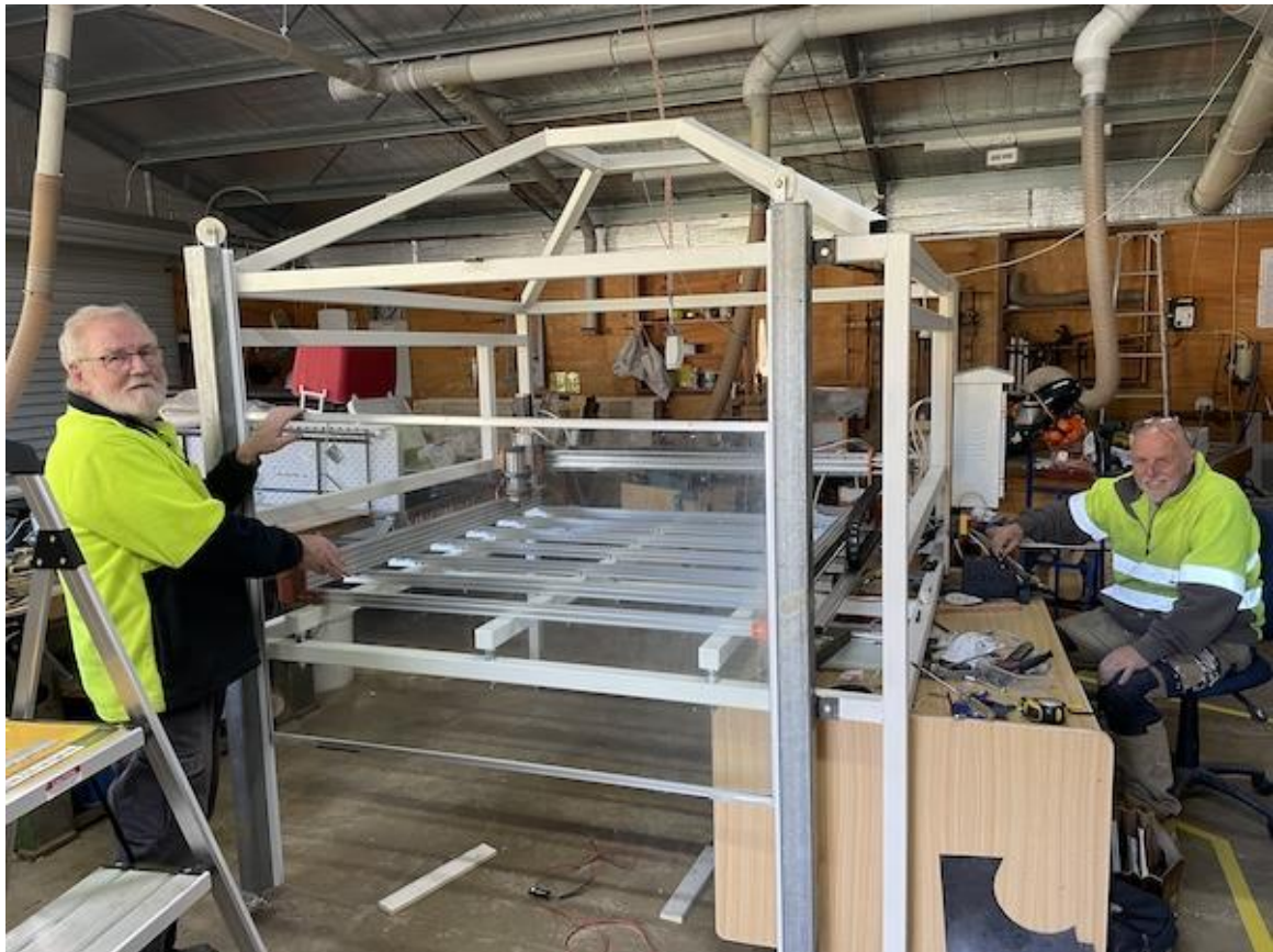
The assembly of our $10,000 CNC Router is progressing well. From left: Mal Darwent who just installed the front window that moves up and down on weights and Pip Armitage working on the electrical and computer set up. Not pictured is Dick Puttyfoot who is also doing a power of work on the electronics side.
